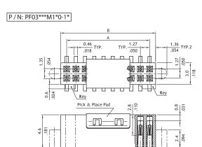
A = 1.27 X No. of Spaces B = A + 1.67C = A + 3.05\* Available in 6 through 100 Circuits
